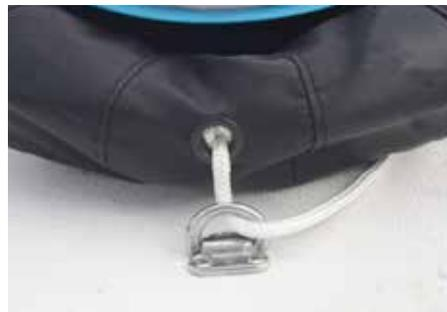
The Frontline of Deckchute is turned in its padeye on the foredeck, and is directed to the pit.
