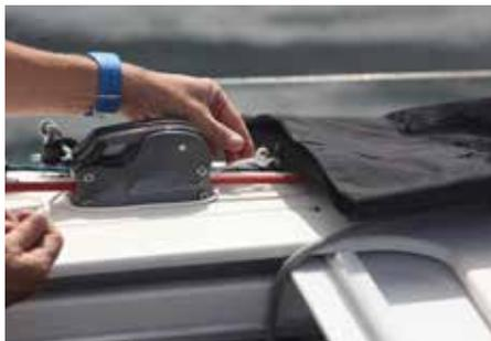
The Pitline of Deckchute is tied to its padeye or to the base of the jammers. It secures the pitend of Deckchute just in front of the jammers.
