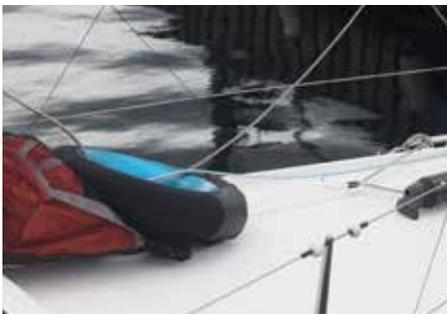
Ready to leave harbour: Deckchute is now in upwind mode. It is lying flat on the foredeck. It is secured by tying the Fidusline, and taking the slack out of the Frontline.
