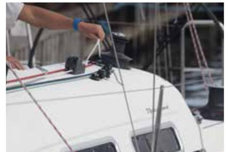
The Frontline of Deckchute is run through its jammer at the pit. Could be the jammer for the 2nd reef.
