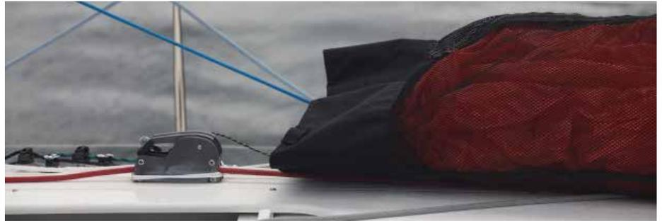
Load the gennaker lying on the foredeck into Deckchute by pulling its Backtail line: In this case the blue line, which is attached to the gennakers tack corner and lower pad by branchlines. Pull it from the cockpit bypassing the brachlines until the gennaker is loaded, resting in Deckchute.
