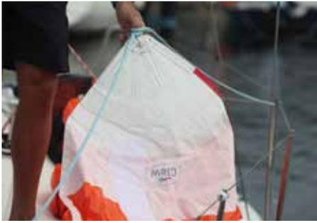
Tie the halyard, the tackline and the sheets to the the gennaker. No hooks, sjackles ect. They will get stuck, tearing Deckchute, and damaging the smooth surface of the Deckchute ring.
