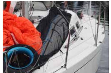
Secure Deckchute to the mast by tying its maststrap. Now it is time to load the gennaker into Deckchute: Unbag it on the foredeck. Pull its Backtail line through the empty Deckchute to the pit.
