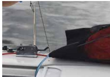
Leaving harbour you may bring Deckchute to "upwind mode": Ease Frontline of Deckchute - open its jammer.
